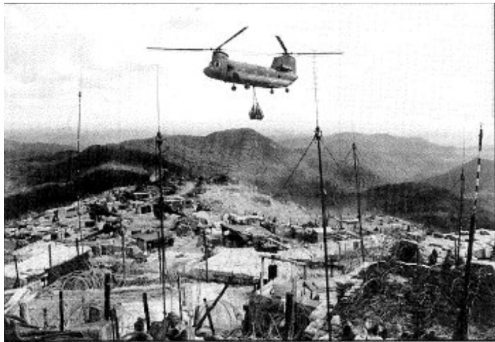
CH-47 Chinook delivering a sling load of supplies to Firebase Ripcord. (Courtesy C. W. Jensen)
